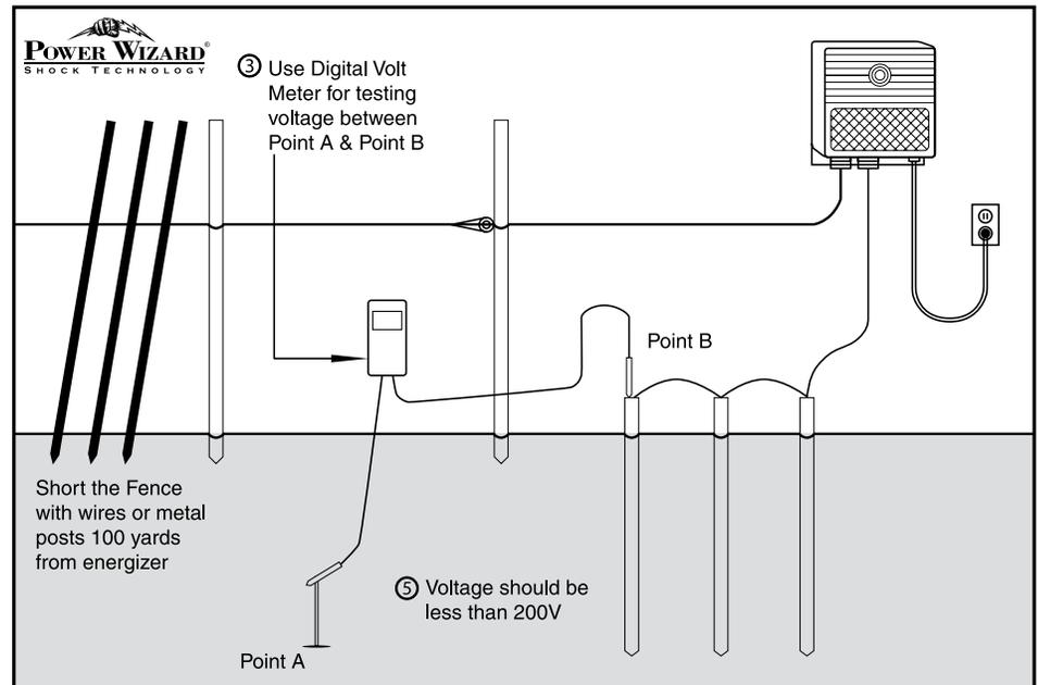
3. Plug the Power Wizard fence energizer in and check the fence line voltage with a digital volt meter. You want to see that the voltage has dropped below 2,000V due to shorting the fence. On some high powered fence energizers you may not be able to short the fence below 2,000V. However, you can still test them at a higher voltage.
